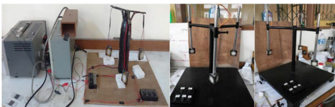
Figure 1: The initial construction of the self-custom-made ultrasound generator (left-most photo) and a modification made to the piezoelectric probe installation (middle and right-most photos).
